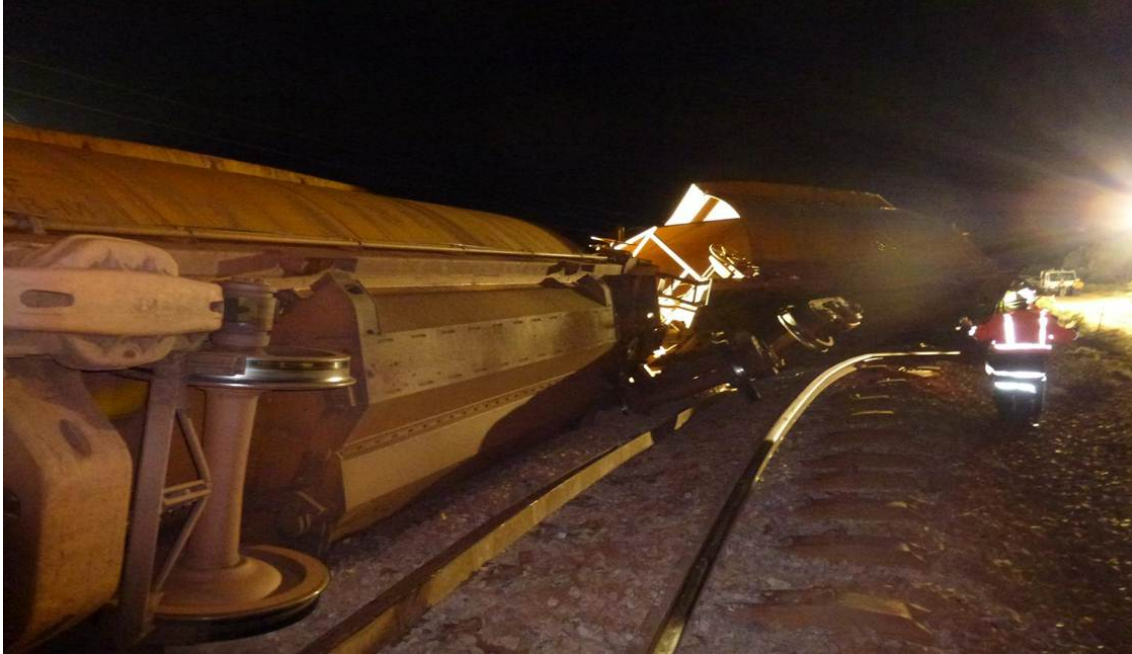
Figure 2: Train 24KW – Derailed Ore Wagons
